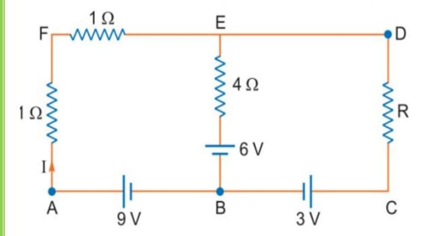
Q12. Using Kirchoff's rules determine the value of unknown resistance R in the circuit so that no current flows through
